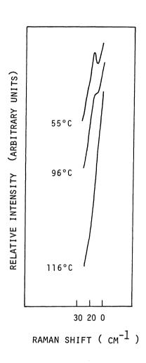
Fig. 1. Raman spectra of TBBA in the crystalline solid phase VIII (55°C and 96°C) and  $S_{\mbox{\scriptsize H}}$  phase V (116°C) on heating.
