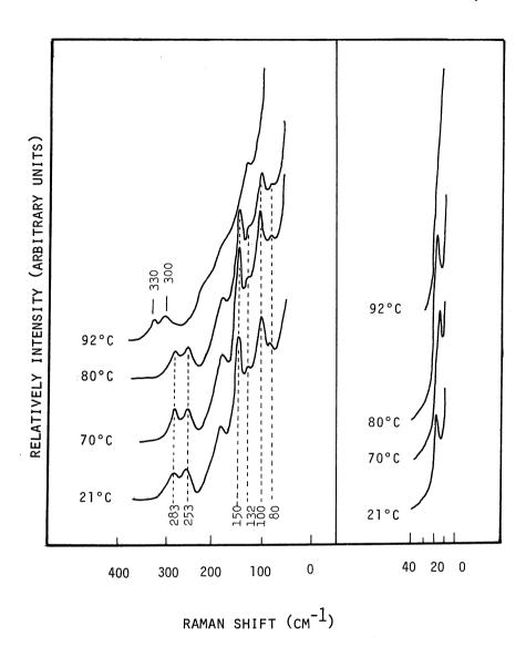
Fig. 3. Raman spectra of TBBA in the  $S_H$  phase V (92°C), phase VI (80°C), phase VII (70°C) and crystalline solid phase VIII (21°C) on cooling.
